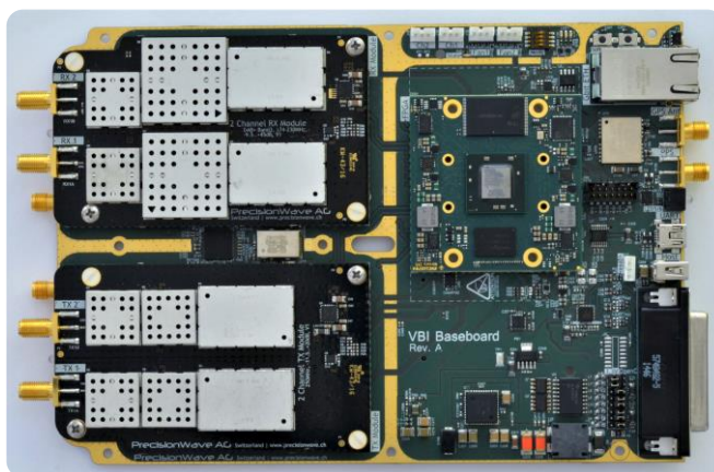
Modular, broadband RF Interfaces (up to 150MHz RX- and 600MHz TX-bandwidth) make our system ready for you customized frequency needs. Contact us with your specifications.
